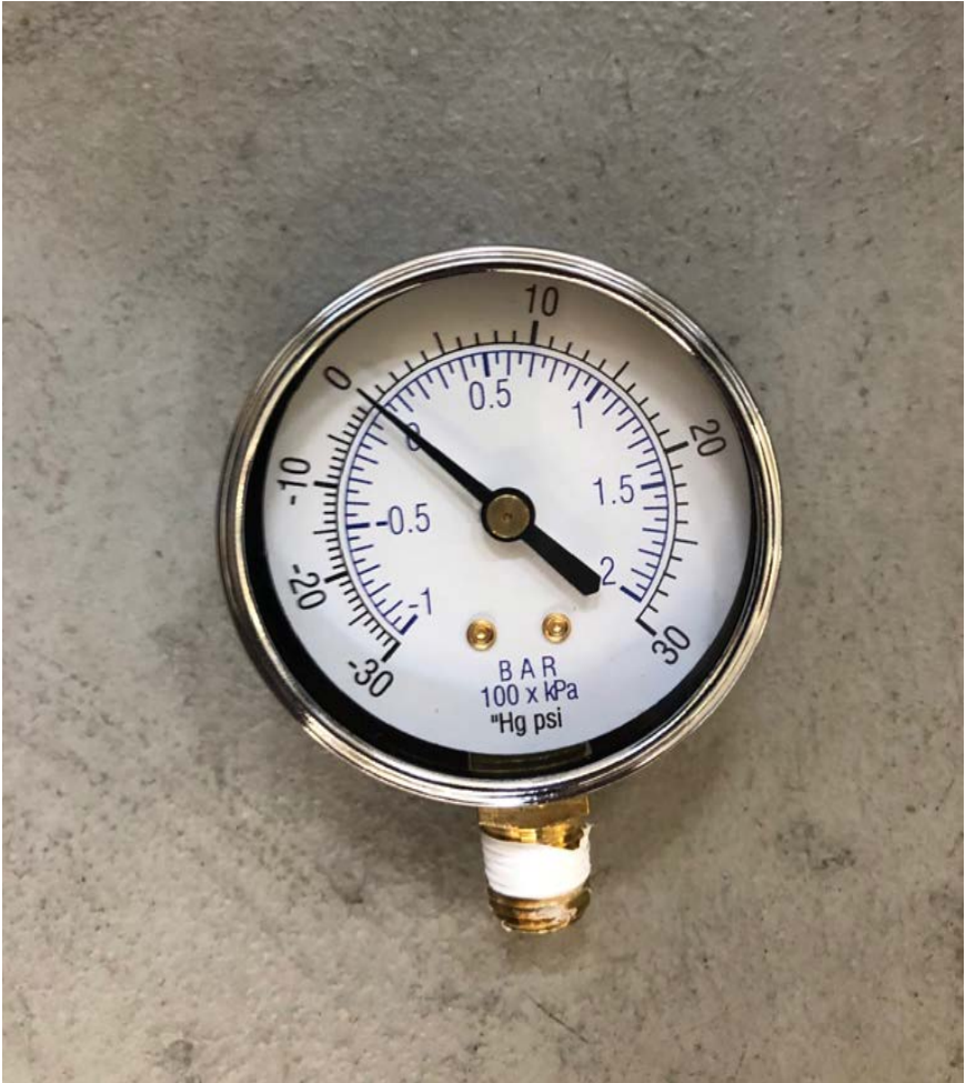
Inlet Vacuum Gauge
