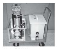
Model #457 For 1 to 10 sumps to 1000 gallons, with heavy oil & solids loading.
