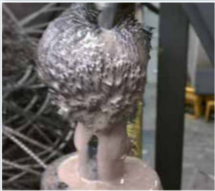
In-Sump Magnet for Chip Control
